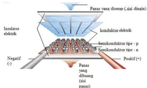
**Gambar 3.** Modul pendingin termoelektrik (Wilsen, S., 2015)
